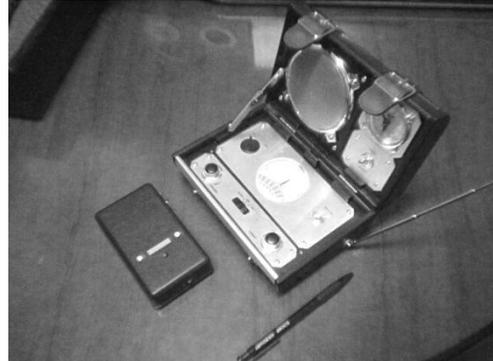
The device masks the real speech signal using a special acoustic noise. It is also used false acoustic signals - transmission FM radio stations.
